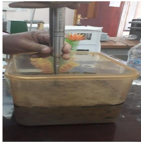
Fig. 9. Undrained shear strength test.
