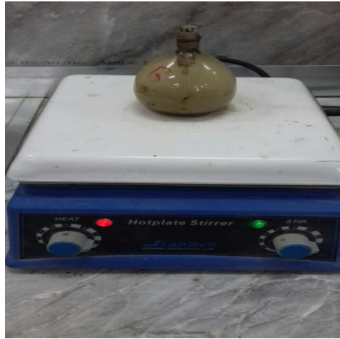
Fig 6. Heating the pycnometer on a hotplate.
