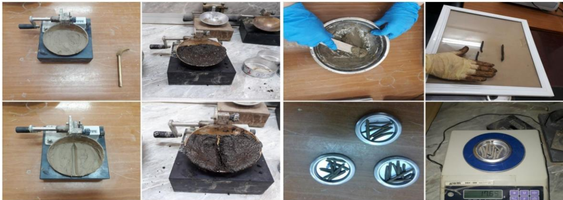
Fig. 5. The Atterberg limits test.
