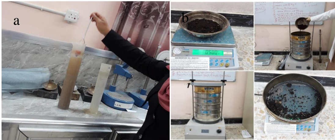
Fig. 4. (a) Hydrometer test (b) Sieve analysis test.
