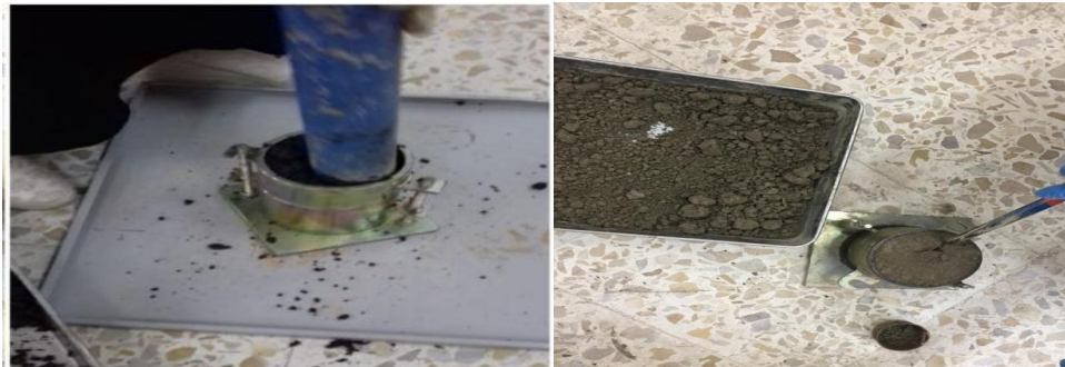
Fig.7. Standard proctor compaction test.
