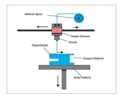
Fig.2. Fused Deposition Modeling (FDM)
