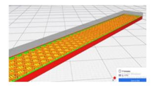
Fig. 4. specimens slicing(RED shill thickness ,Orange infill pattern,Green layer thickness)
