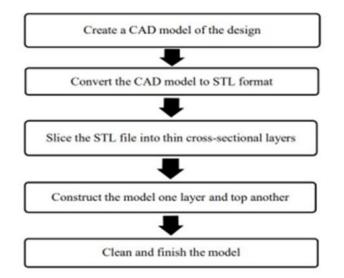
Fig.1.steps of rapid prototyping
