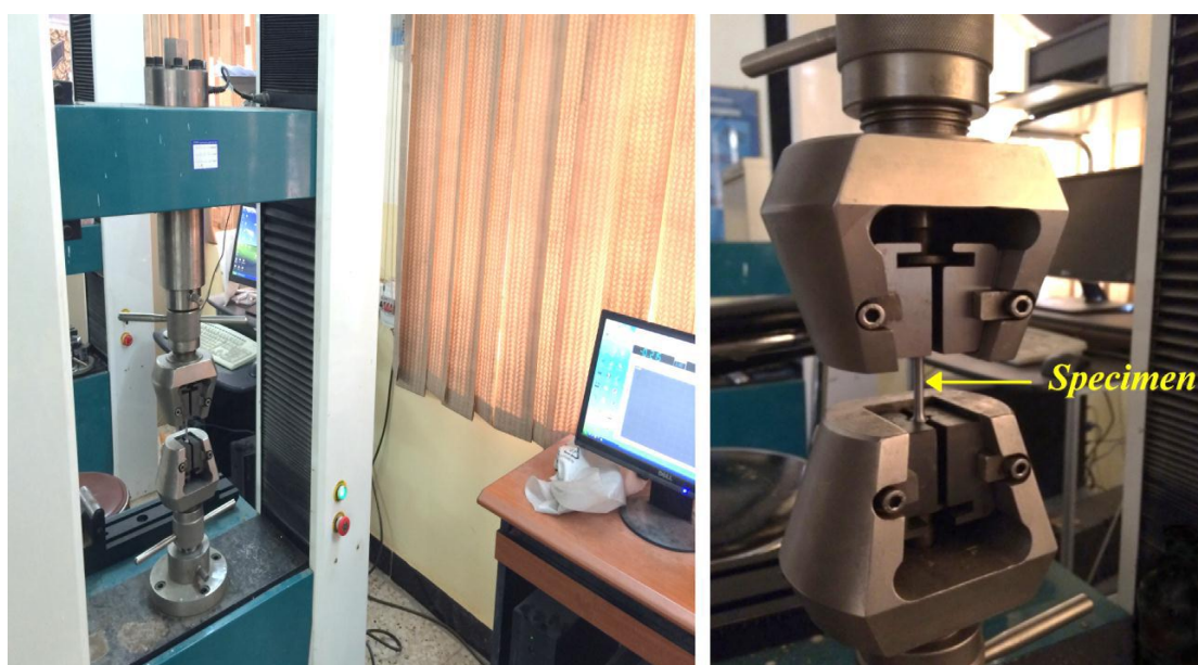
Figure (3) :Tensile test machine WDW-200E.
